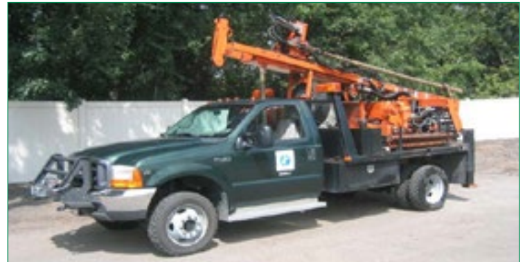
Soil boring equipment mounted on a truck.
